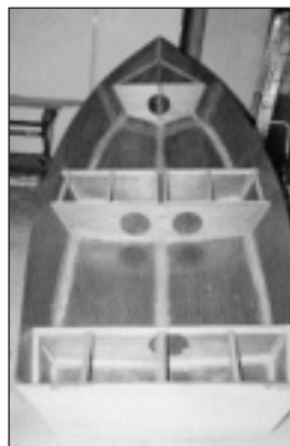
WITHOUT the seat tops to show the bracing and the centreboard box
