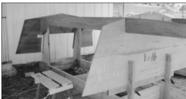
FRAMES and stringers on jig.
