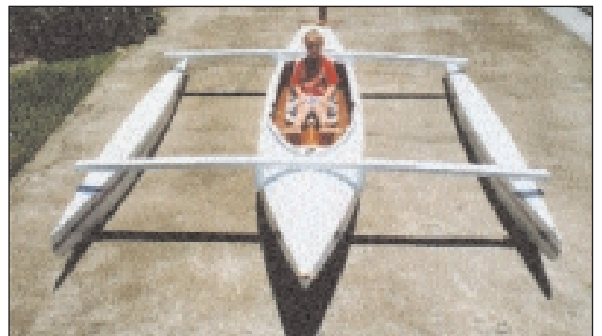
from left to right: 16ft kayak ready to paddle, although my granddaughter may have to grow a bit; add the crossbeams with 4 x s/steel bolts; add the pontoons with 8 x s/steel bolts.
